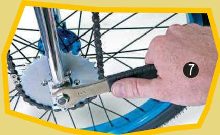
Finally, tighten the axle-screws equally and step by step on both sides to fix the wheel in the frame. (7)
